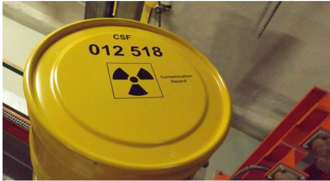
Container with cemented waste
