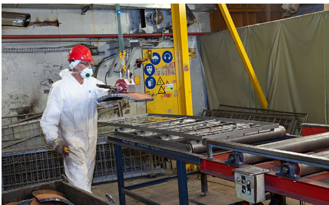
Decontamination unit for dismantled equipment
